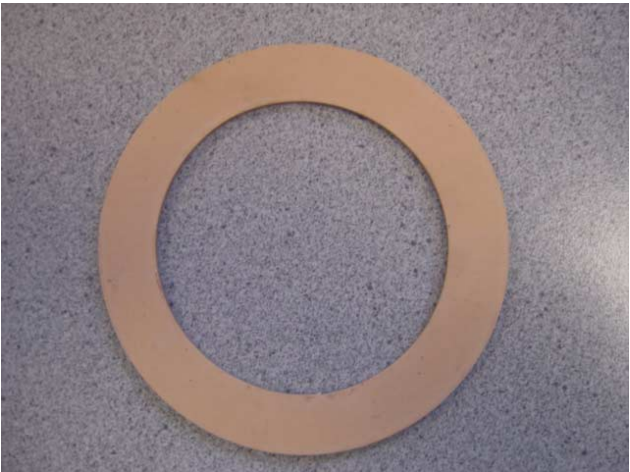
Photo 1 - Gasket before test - TEADIT - 1590 - 5" OD * 3.5" ID - thickness:1/8"
