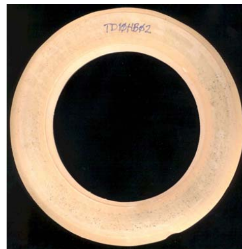
Photography 3 Tested gasket sample TD10HB02
