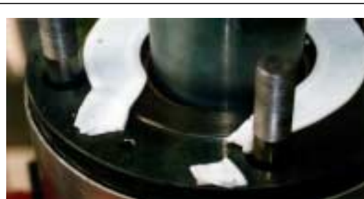
HOBT rig – PTFE Gasket Blow Out example
