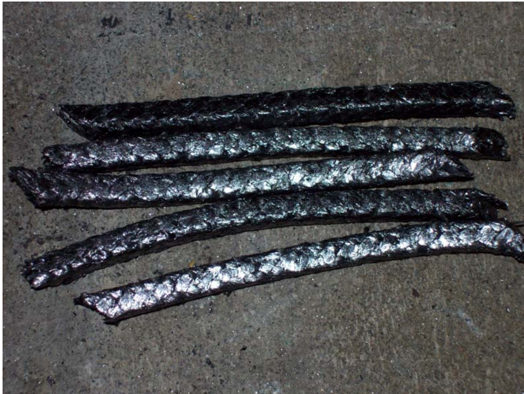
Packing rings cut from spool by Yarmouth prior to test
