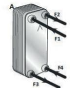
HCBPs with UL approval for use with CO<sub>2</sub> according to UL files section II or VI. When used with CO<sub>2</sub>, the system should include a pressure 2 relief valve on each side of the HCBP. The pressure relief valve must open if the system pressure reaches 0.9 × design pressure.
