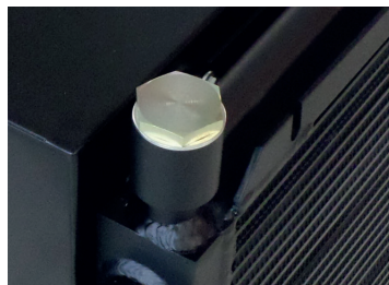
Externer Bypass External Bypass
